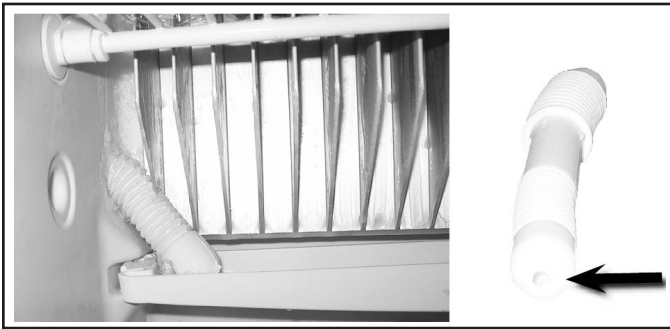
Check orifice diameter. Should be 1/4"
