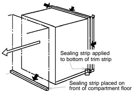
**NOTE:** Be careful not to damage the sealing strip applied to the floor of the enclosure when the refrigerator is put in place. The refrigerator is secured in the enclosure with six screws and they must be installed in the following order:
