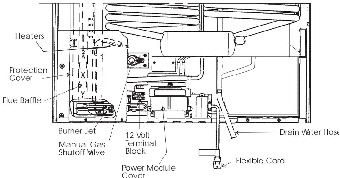
plug. The free length of the cord is 2 feet and therefore recommended that the receptacle be located to the right side of the refrigerator (viewed from the rear) and approximately 6 inches from the floor (see FIG. 7). This allows easy access through the vent door. The cord should be routed to avoid direct contact with the burner cover, flue cover or any other components that could damage the cord insulation.
