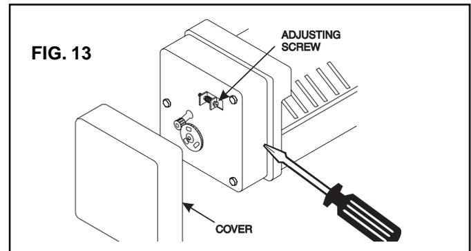
**CAUTION: DO NOT** turn the screw more than one turn at a time. The ice maker should be allowed to cycle several times before another adjustment is made. Be sure to replace protective cover on the cycle after adjustments have been made.
